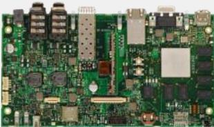
The Viper boards from Barco Silex are fully integrated boards that enable the development of ultra-low latency audio/video over IP products. The video stream is compressed with VC-2 HQ and enables up to 4K HDMI over a single 1G Ethernet cable.
